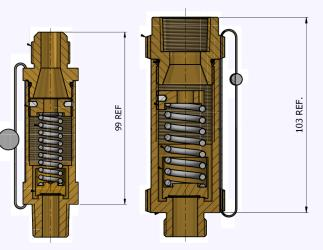
Maximum permissible built up back pressure = 10% of set pressure at or below which flow is not reduced. Stable operation on flows down to 50% of valve rated capacity.
