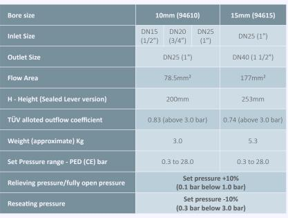
• TÜV alloted outflow coefficients for pressures above 3.0 bar, for lower pressures please see the flow rate tables or contact Seetru.
