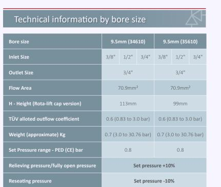
Maximum permissible built up back pressure = 10% of set pressure at or below which flow is not reduced. Stable operation on flows down to 50% of valve rated capacity.
